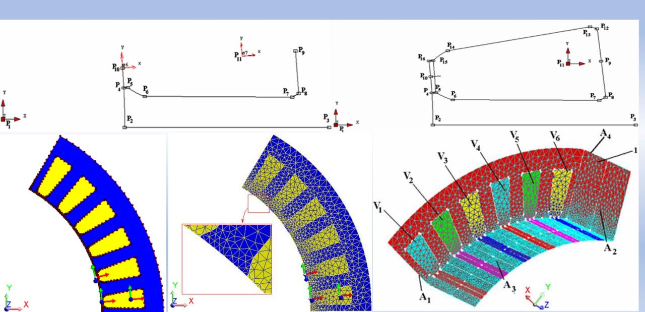
THE CONSTRUCTION OF THE 3D PARAMETRIZED GEOMETRY OF THE ROTOR CORE IN CATIA V5 R 17 (Full core rotor with 12-poles and the 3D computing domain has a pair of poles 44,15 LIM1
