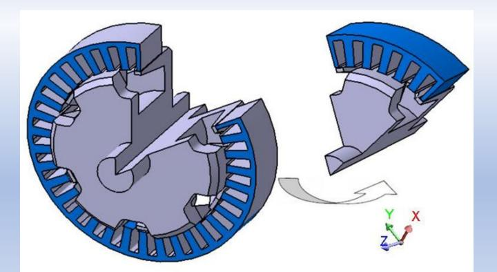
THE CONSTRUCTION OF THE 3D PARAMETRIZED GEOMETRY OF THE STATOR CORE IN PREFLUX 3D (Full core stator with 36 slots and 3D computing domain has 6 slots
